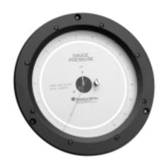
For routine test and production uses, this capsule-type gauge offers an acceptable balance among size, readability, accuracy, and price. Available in 18 standard ranges (including vacuum and compound ranges), the Series 300 is convenient to use. Pressure is applied to the capsule through a single connection in the case. Readings are referenced to atmospheric pressure in the case.
